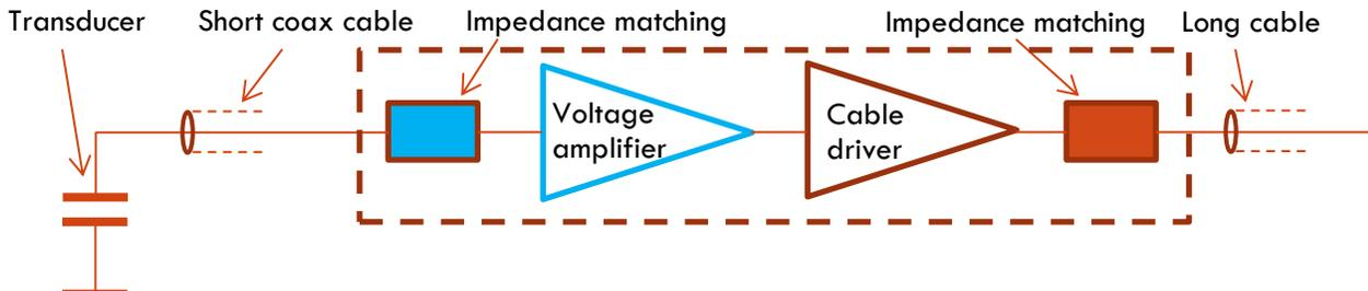
**FIGURE 6: PARTS OF A PREAMPLIFIER**
