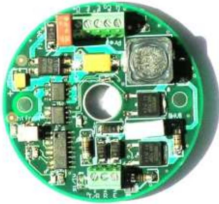
**FIGURE 7: PULSER PREAMPLIFIER (WITH MORE ELECTRONICS ON THE BACK)**
