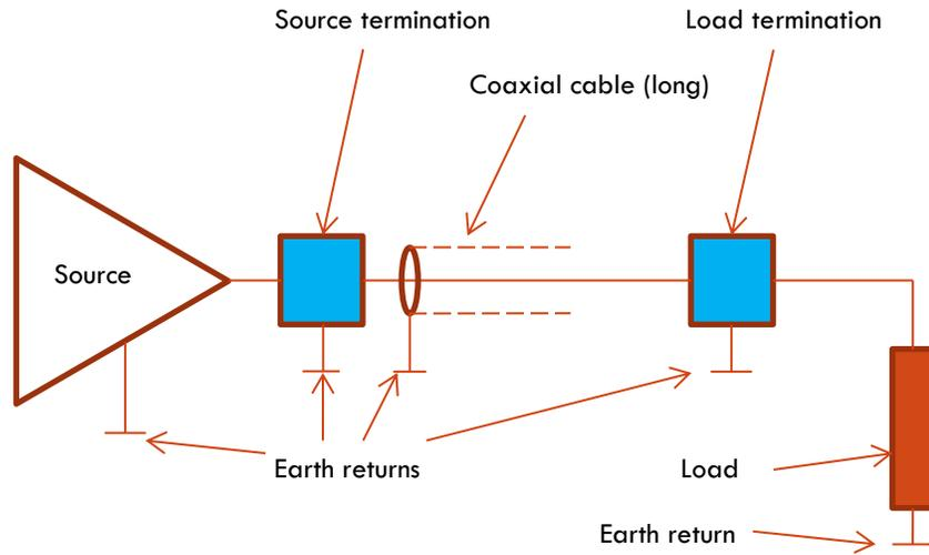
**FIGURE 1: CABLE TERMINATION**
