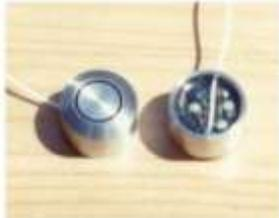
**FIGURE 5: AE SENSORS WITHN PREAMPS**
