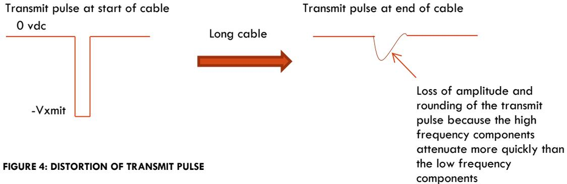
**FIGURE 4: DISTORTION OF TRANSMIT PULSE**
