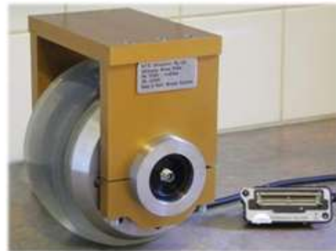
Modified PL180 holding a single PA transducer
