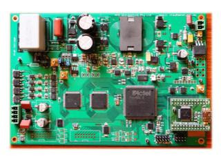
NTS Ultrasonics Pty Ltd designs ultrasonic instrumentation for non-destructive testing and similar applications. Recent designs are of the "black box" type with all function control carried out from an external computer or microprocessor. Circuits have been developed with SPI, USB 2.0, and gigabit Ethernet communications interfaces.
